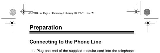
Plug one end of the supplied modular cord into the telephone line's modular jack. Then plug the other end into the ET-153's TEL. LINE jack.
